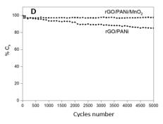
Figure 5: (A) GCD curves of rGO/PANi and (B) rGO/PANi/MnO<sub>2</sub>; (C) variation of specific capacitance with current density; (D) capacitance retention of rGO/PANi and rGO/PANi/MnO<sub>2</sub> electrodes after 5000 cycles at 15 A/q
