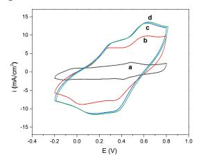
Figure 3: CV curves of (a) rGO/PANi and rGO/PANi/MnO<sub>2</sub> electrodes with deposition times of (b) 100 s, (c) 200 s, and (d) 300 s in 1 M H<sub>2</sub>SO<sub>4</sub>.
