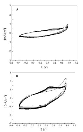
Figure 1: CV curves recorded on GO/ANi printed electrodes in 0.1 M H<sub>2</sub>SO<sub>4</sub>: (A) without GO reduction, (B) after 30 s of GO reduction
