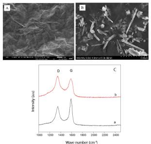
Figure 4: FE-SEM images of (A) rGO/PANi and (B) rGO/PANi/MnO<sub>2</sub> films, (C) Raman spectra of (a) GO/ANi and (b) rGO/PANi/MnO<sub>2</sub>
