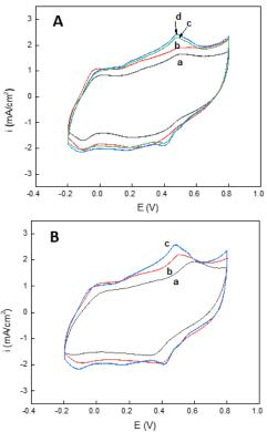
Figure 2: CV curves of rGO/PANi electrodes synthesized with different: (A) GO reduction times: (a) 10 s, (b) 20 s, (c) 30 s, (d) 40 s and (B) GO: ANi ratios in  $1 \text{ M H}_2\text{SO}_4$ : (a) 2:1, (b) 1:1, (c) 1:2.
