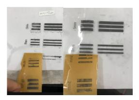
Figure 1. Images of conductive ink with 1% PVP (a) and 3% PVP (b) after a single tape-peel test
