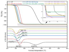
Fig 5: Comparison of AP decomposition promoted by Fe<sub>3</sub>O<sub>4</sub>/CuO nanocomposites based on GO, rGO, and graphene (adapted from previous research [11])
