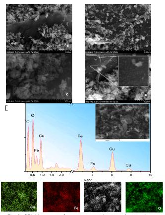
Fig 3: SEM images of nanocomposites synthesized on GO (A), rGO-200-1.5 (B), rGO-200-4 (C), and rGO-250-4.5 (D) substrates; with the EDX elemental mapping of the nanocomposite sample based on rGO-250-4.5 (E)
