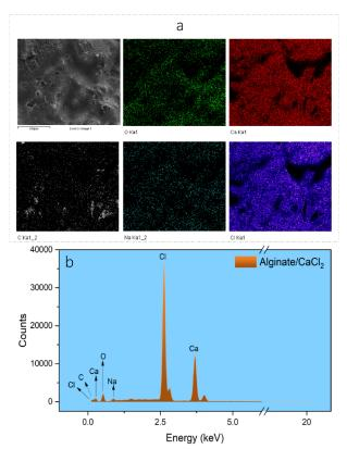
Fig 5: Mapping scan images (a) and EDX data (b) of Alginate/CaCl<sub>2</sub>
