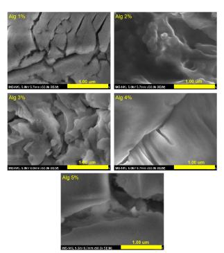
Fig 2: SEM images of Alginate/CaCl<sub>2</sub> composite
