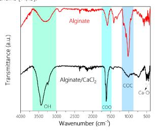
Fig 4: FTIR spectrum of Alginate and Alginate/CaCl<sub>2</sub> composite
