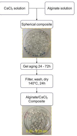
Fig 1: Synthesis scheme of the Alginate/CaCl<sub>2</sub> composite
