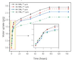
Fig 6: Water vapor adsorption kinetics of the Alginate/CaCl<sub>2</sub> composite at RH 70% and RH 90%, showing performance during the 1<sup>st</sup> cycle and after regeneration
