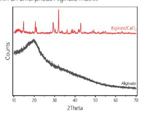
Fig 3: XRD pattern of Alginate and Alginate/CaCl<sub>2</sub> composite
