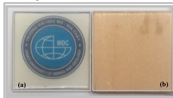
Figure 2. Images of Transparent wood sample (a) fabricated from balsa wood (b)
