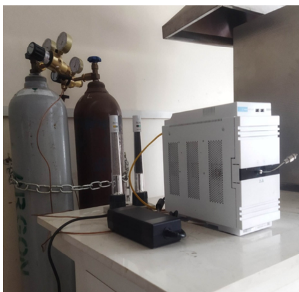
Fig. 2: Setup of the Macro-GC 900 for syngas analysis
