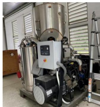
Fig. 1: The commercial downdraft fixed-bed gasifier (PP20 All Power Lab)
