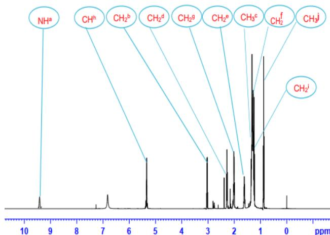
Figure 3:  $^1\text{H NMR}$  of IL triethylammonium oleate obtained by 3 step method
