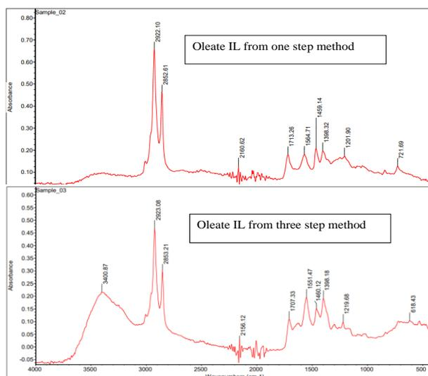
Figure 1: FT-IR spectra of IL triethylammonium oleate obtained by one step and 3 step methods
