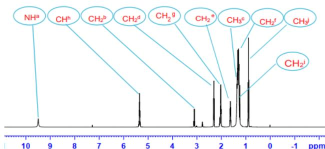
Figure 4: <sup>1</sup>H NMR IL triethylammonium oleate by one step method
