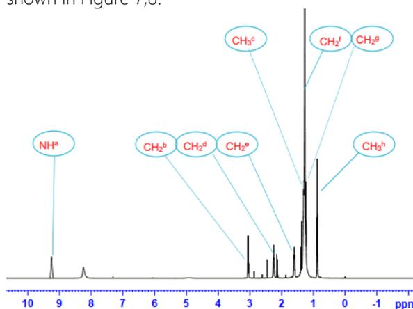
Figure 7: <sup>1</sup>H NMR of IL triethylammonium stearate by 3 step method
