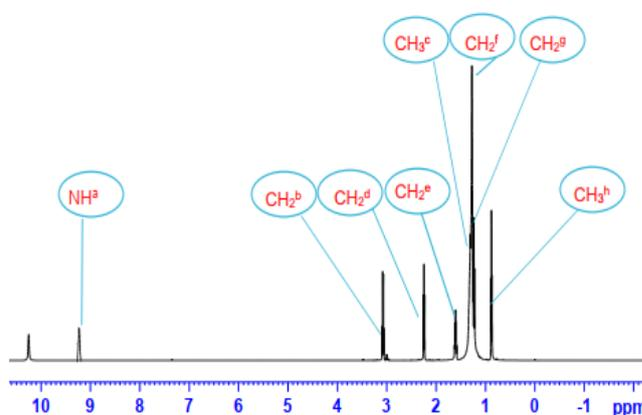
Figure 8: <sup>1</sup>H NMR of IL triethylammonium stearate by one step method
