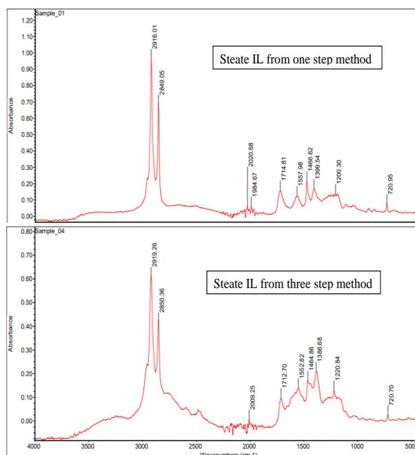
Figure 6: FT-IR of IL triethylammonium stearate
